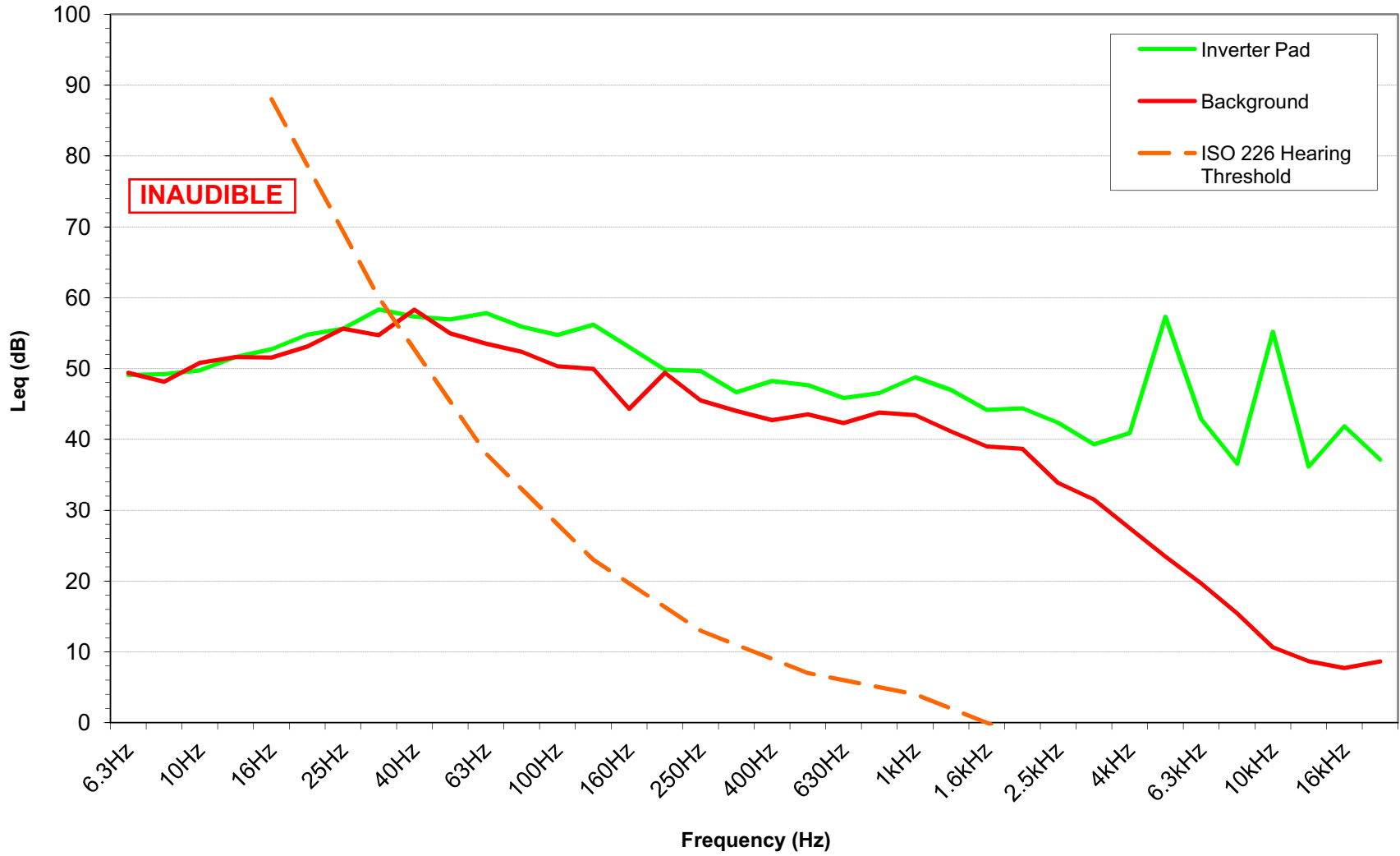
Figure 8. Frequency Spectrum of Sound Levels (Leq) at a Distance of 10 Feet from the Inverter Pad at Site #2
